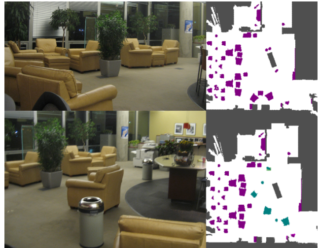
Fig. 1. A situation that requires an object based map. The top image represents the initial configuration of the map. The bottom image is the same map, with the furniture re-configured. By using an object-based map, the robot was able to rearrange the furniture in it's own map to match the real world. The robot accomplished this task by noticing which objects were no longer where the static map indicated, and point-matching those objects to objects it observed. In addition, the robot labeled the moved furniture, as well as furniture in the map that looked similar, as movable.
