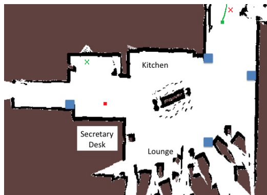
Fig. 1. A hindrance-sensitive robot path planning problem in our experimental environment containing a person (green square) in the upper right with a previous trajectory (green line) and intended destination (green X) near a doorway, and a robot (red square) near the secretary desk with its intended destination (red X) near the person’s starting location. Robot-person hindrances are likely if the person and robot both take the distance-minimizing path to their intended destinations.
